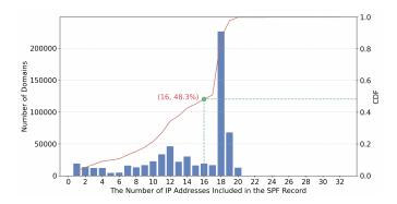
Fig. 7. IP Coverage Analysis of SPF Records. The x-axis represents the number of IP addresses included in the SPF records, calculated with the  $log_2^{number}$  function. For example, 51.7% of domains have SPF records that contain more than 65,536 (2<sup>16</sup>) IP addresses.
